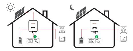
**Energy flow:** PV and Battery  $\rightarrow$  Load
