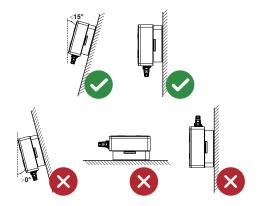
• Leave the enough space around inverter, easy for accessing to the inverter, connection points and maintenance.
