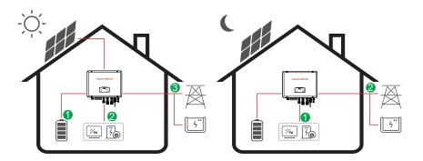
**Energy flow:**  $PV \rightarrow Battery \rightarrow Load \rightarrow Grid$
