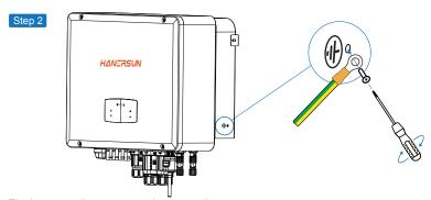
Fix the grounding screw to the grounding connection of the machine housing.
