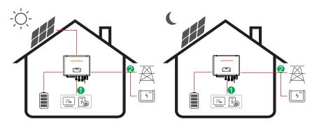
**Energy flow:** Battery and  $PV \rightarrow Load \rightarrow Grid$
