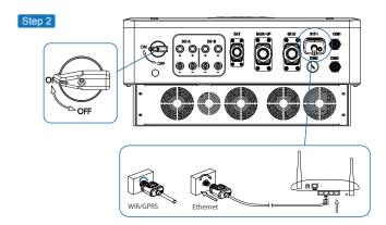
Turn on the DC switch and AC circuit breaker, and wait until the LED indicator on the monitoring module flashes, indicating that the monitoring module is successfully connected.
